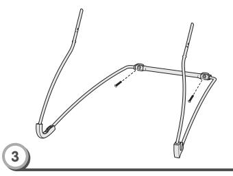
• Insert an M5 x 20 mm screw through each foot and tighten.
